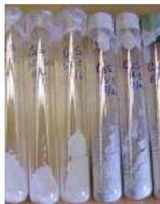
Figure 1 Nano-cement samples
