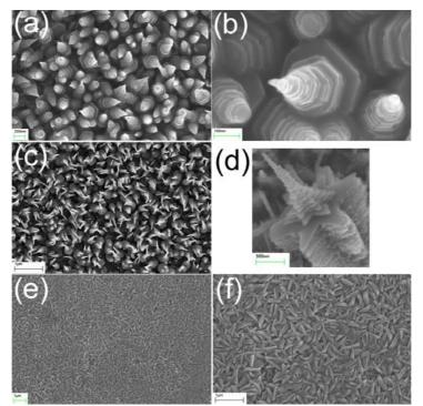
ZnO nanostructures from solution growth methods.
