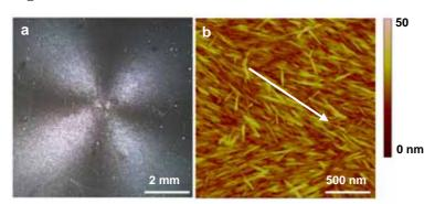
The orientation of cellulose nanocrystals can be seen on many length scales. a) Polarized-light microscopy image of LbL films of (PAH/cellulose)<sub>10</sub> b) tapping mode AFM height image of the same film.
