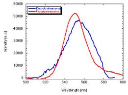
Electroluminescence spectrum (blue) of a HST-LET biased at Vds = Vg = - 60 V and photoluminescence spectrum (red) of the same film
