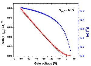
Transfer characteristics of a HST-OFET (deposition rate = 0.2 A°/s, nominal thickness = 18 nm, W/L=18800/40  $\mu$ m/ $\mu$ m)
