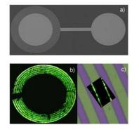
Optical images of: a) Interdigitated bottomcontact device b) Green electroluminescence of HST-LEFT c) magnified contacts and localized light emission
