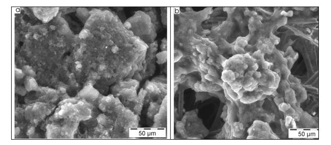
**Figure1.** Scanning electron microcopy images of biofilm growth on: a) carbon aerogel and b) MWNT
