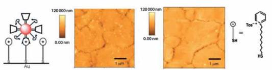
Specific binding of the calixarene-modified gold nanoparticles, from aqueous solution to a self-assembled monolayer (SAM) of the pyridinium salt on a gold surface shown by AFM (left). The control experiments (right) show the nonspecific attachment of only very few particles to the SAMs.
