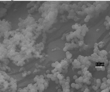
Fig. 2. Scanning electron microscopy image of PS-VBC-DVB with nanoparticles loaded at 1% by mass to the amount of monomer.
