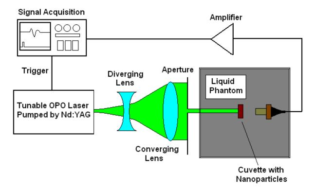
Optoacoustic Spectroscopy measurement scheme composed using tunable Nd:YAG laser for gold nanoparticle characterization in a liquid phantom representing human soft tissue
