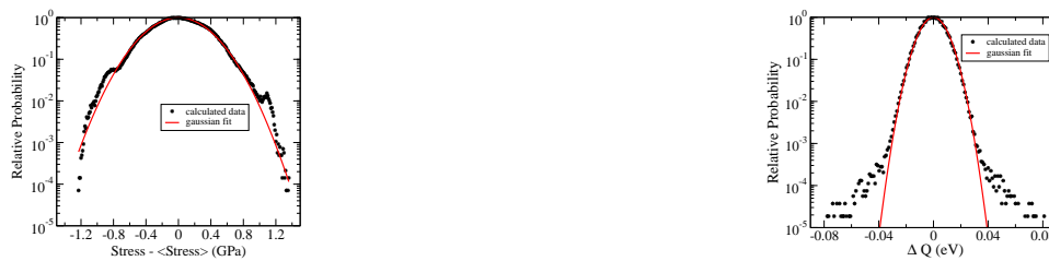
FIGURE 3: Probability distributions of the engineering stress and the heat evolved ( \Delta Q ) in the non-linear (plastic) regime derived from molecular dynamics calculations on aluminum nanowires, containing 463 atoms, stretched at a constant strain rate. The distribution contains more than 1.5 million counts (1500 realizations by at least one thousand points along the stress-strain curve). The (red) continuous curves are Gaussian fits to the numerical data over the stress range [-0.5, 0.5] GPa or the heat range [-0.02, 0.02] eV.
