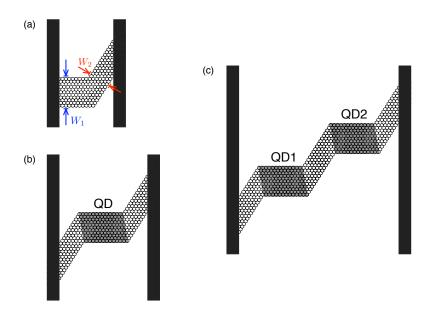
**Graphene nanoconstrictions** with zigzag edges studied in the present work. 120-degree kink (a) blocks the current at low bias for  $W_1 \neq W_2$ . Double kink (b) traps an electron in the *shadow* area and thus operates as a single-level quantum dot, whereas constriction with four kinks (c) operates as a double quantum dot. Each of the devices is connected to heavily-doped graphene leads marked with the dark bars.
