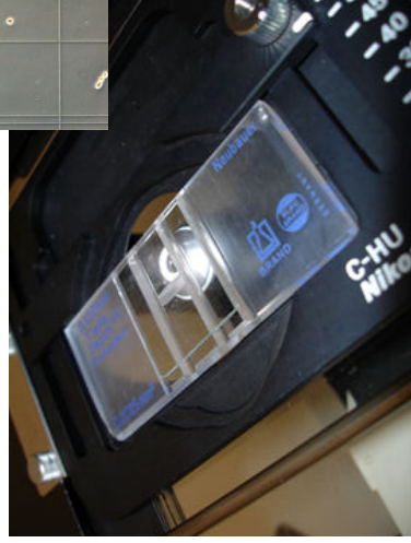
cell counting with an hemocytometer
