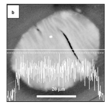
Nickel distribution obtained by energy dispersive spectrometry in the section of a particle. The noisy line represents the nickel content. The continuous line represents the selected line for analysis and the discontinuous line represents saturation of the signal. Bar length =  $20 \mu m$ .
