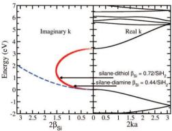
Complex band structure for silicon hydride chains and silane-based tunnel junctions with amine or thiol linkers. The decreased HOMO-LUMO gap size in the silanes, compared to the alkanes, makes the values decay constant for silanes more sensitive to small differences in the Fermi-level alignment compared to alkanes.
