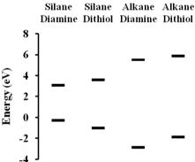
Molecular frontier energy levels for the hexane and hexasilane bonded to gold clusters via amine and thiol end groups. Energies levels are approximated by the Kohn-Sham eigenvalues from the DFT B3LYP calculations. The zero of energy is taken to be the Fermi level approximated as the work function of gold (-5.1 eV).
