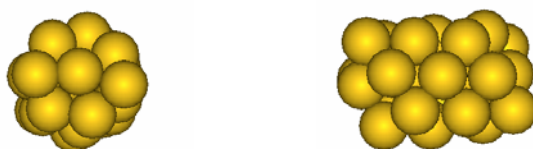
Fig.1. Snapshot of a 7-fold nanowire segment resulting from the coalescence of two Au 13 clusters. Views parallel and perpendicular to the axis of the (8,8) CNTs are displayed. The CNTs is not shown.
