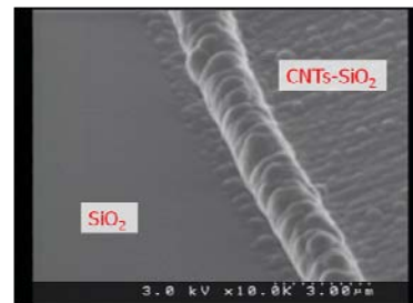
Figure 4. SEM image of CNTs-SiO 2 . The CNTs aligned on the SiO 2 surface are buried into SiO 2 using ozone-TEOS CVD.
