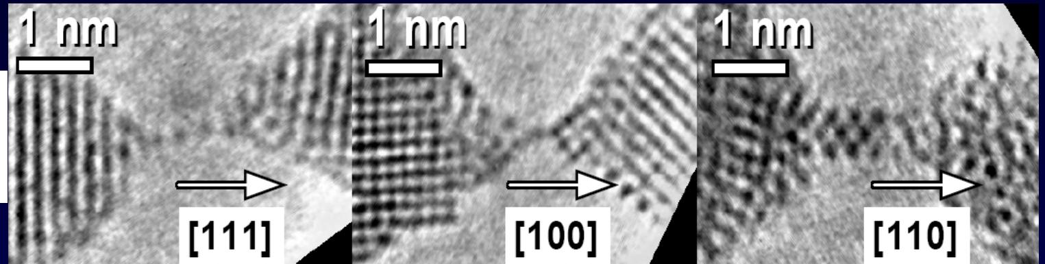
A **New** Tubular Structure of [100] NW is observed at **RT** and **LT**
