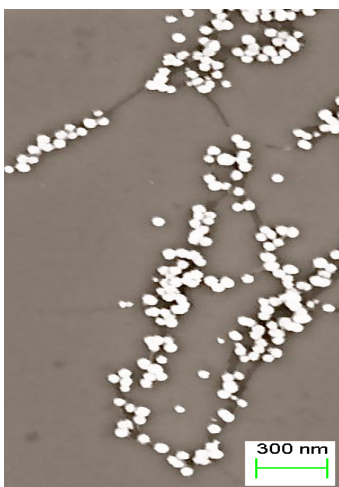
Figure 1: Ni deposited on TMV via electroless deposition
