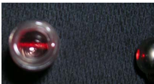
Figure 3. The Tyndal scattering in a solution of PVA-Perylene containing dispersed few layer graphene
