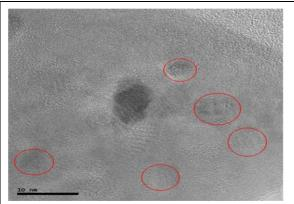
**Fig. 2:** Crystalline nanoparticles obtained by laser ablation of fish bones in de-ionized water.
