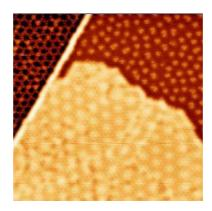
STM picture (40x40 nm², -1.0 V, 0.9 nA, 77 K) of the surface of epitaxial graphene obtained after gold deposition. It shows the pristine monolayer graphene and two new domains due to the intercalation of gold atoms between the monolayer graphene and the buffer layer. The first domain consists in the intercalation of gold clusters and the other one is formed by a freestanding monolayer of gold [4].
