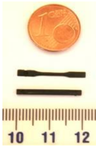
Fig. 1 - Microinjection moulded composite specimens: a) tensile and b) impact.
