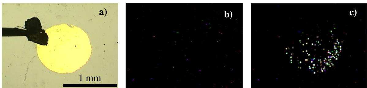
Figure 2. EL points under reverse voltage : (a) image of the electrode; (b) reference at 0V; (c) EL at -18V, -2.7 A/cm 2
