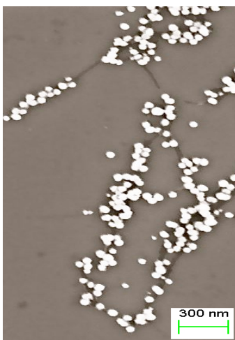
Figure 1: Ni deposited on TMV via electroless deposition
