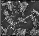
These samples contain a large number of nanowire structures together with abundant globular formations of PPy. It should be remarked that the metallic copper core is single-crystalline in nature as showed by the SAED pattern.
