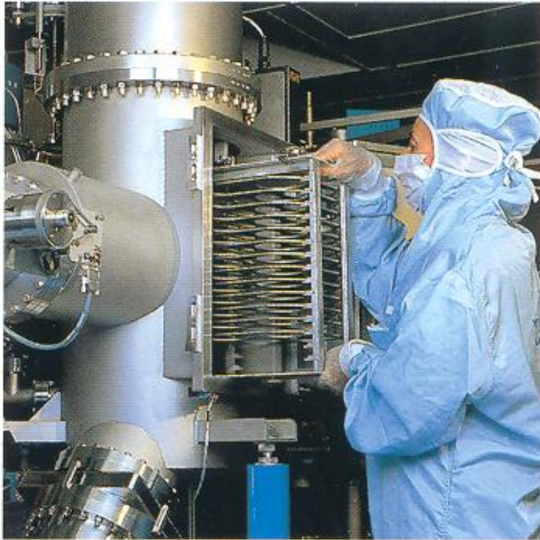
Unloading a cassette containing sixty four-inch epitaxied aluminum gallium arsenide wafers.
