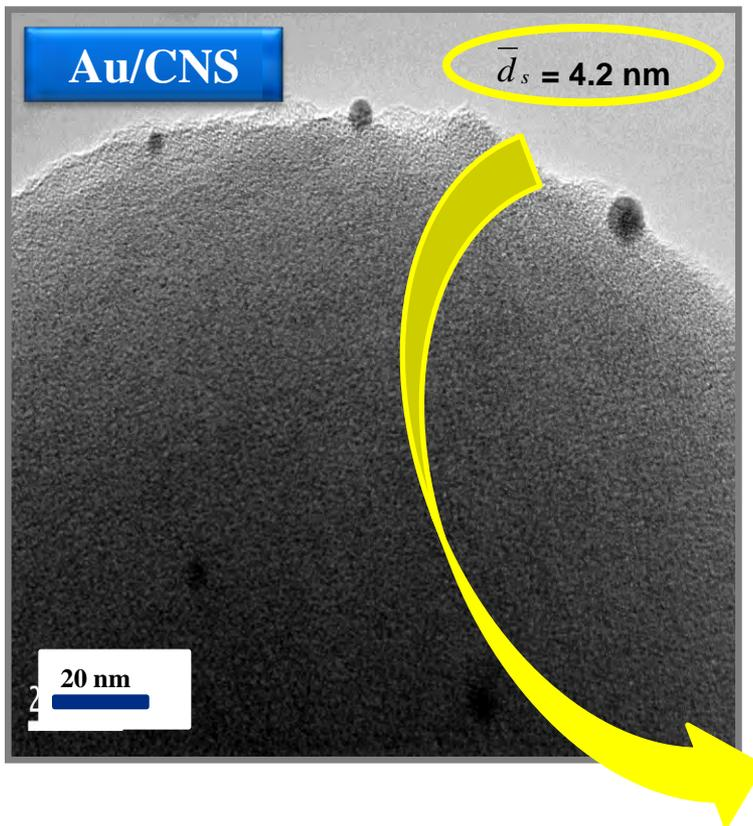
The graphite sheets are not closed shells but rather waving flakes that follow the curvature of the sphere, creating many open edges at the surface that give the structure a high chemical reactivity.
