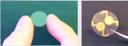
**Basis: Quartz blanks (AT-cut), 168 μm thick**
