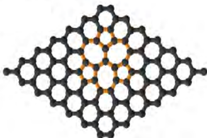
Divacancy 555777 3-fold symmetry axis
