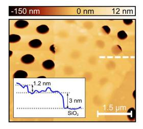
**Figure 1.** Contact mode AFM topography of a 3-4.2 nm thick MoS2 flake (5-7 layers thick). (inset) Topographic line profile acquired along the dashed line.
