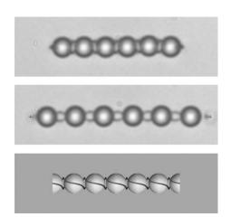
Fig. 2. Nematic colloidal wire, assembled from 2.3  $\mu m$  silica microspheres in a nematic liquid crystal 5CB. The microspheres are bound together by entangled defect lines, which are wrapped around the microspheres. The bottom image shows the results of Landau-de Gennes simulations.
