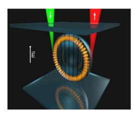
Fig.4 A single droplet of a cholesteric liquid crystal doped with a fluorescent dye and immersed in water or other immiscible liquid is a 3D microlaser. Because of chirality, the LC molecules form a helical birefringent structure, originating at the center and spiraling to the surface. Optically, this is a spherical, onion-Bragg microresonator. When pumped with external light, the 3D microlaser starts emitting coherent light in 3D.
