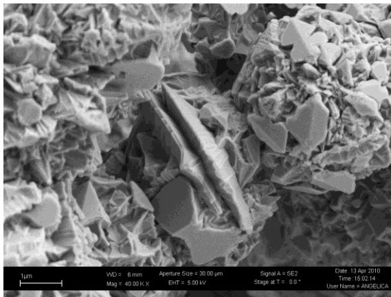
Fig1. FESEM image of the nickel particles. The scale bar corresponds to 1 μm.
