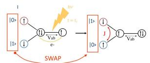
This molecular logic gate would be made of Ruthenium (III) and (II) metal centers [3,4,5], which magnetic interaction could be turned on/off by changing the oxidation state of the central molecule using an appropriate light radiation.
