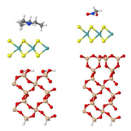
**Left panel:** a triethylamine (TEA) molecule on top of the  $MoS_2$  monolayer on a silanol substrate **Right panel:** a nitromethane (NM) molecule on top of the  $MoS_2$  monolayer on a siloxane substrate
