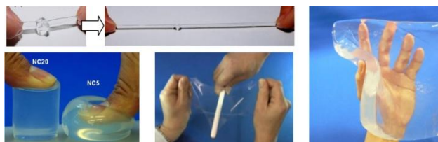
Figure 1. NC gels with various sphaes, e.g., rod, bulk, film, sheet, and deformations such as knotted and stretched NC gel, compression of NC gels with different clay content, and strong resistance against bar-pushing by a thin film of NC gel.
