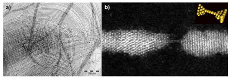
Figure 1. a) TEM and b) HAADF-STEM images of Au NWs. Single-atom thick chain formed during wire fragmentation under E-beam irradiation.
