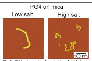
Fig 2. PG4 adsorbed at low (left) and high (right) salt levels. At low salt level, the electrostatic repulsion between the charged groups on the dendrons results in a more stretched configuration.
