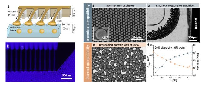
Fig. 1 (left): Schematic of a step emulsification channel arranged with parallelized droplet makers (a) and an actually working device producing monodisperse oil-in-water droplets (b).
