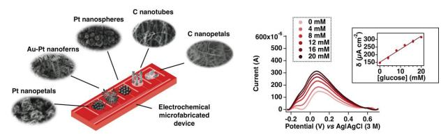
Multisite electrochemical sensor including microelectrodes modified with CVD carbon nanomaterials and template-free electrodeposited Pt and Au-Pt nanoporous layers (left). Electrochemical measurements of different concentrations of a metabolite (glucose) and relative calibration curve (right).
