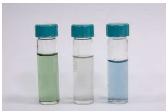
Figure 1. The MoO x nanoparticles produced from 60 mg/ml of MoS 2 in (from left) NMP, water, 45% ethanol in water.
