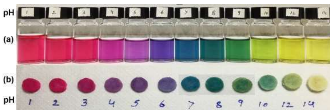
Figure 1. (a) Anthocyanin solution response upon pH changes (b) Anthocyanin treated PVA/Cellulose foams upon pH changes
